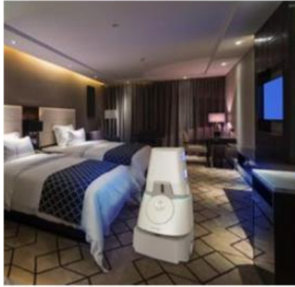
Robot sanitizes in-room high-touch surfaces such as light switches, door handles, remote controls, nightstands, and bathroom surfaces.
